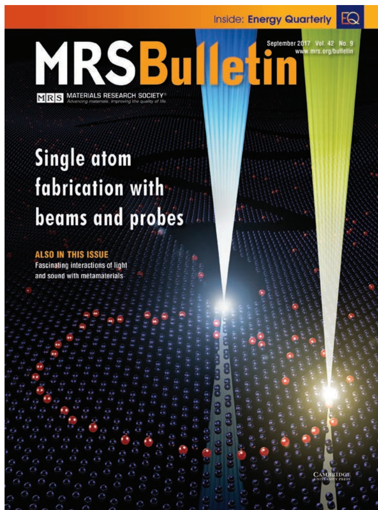
Journal cover showing an artistic rendering of scanning transmission electron microscope-based single-atom-level manipulation and fabrication of 2D materials. Electron beams can be used to cut or remove material and control the position of atoms and dopants on or within a lattice. Image credit: ©2017 Materials Research Society
